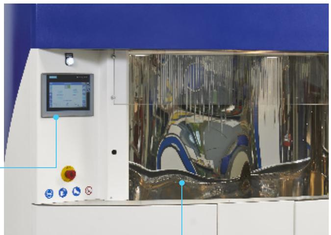
Super mirror finish stainless steel extraction enclosure (Ra = 0.02  $\mu\text{m}$  max)
